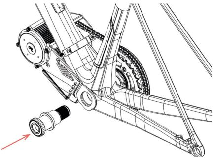
4. Insert the spindle from the right (drive). Note that you will need to line up the splines with the chainring assembly. If your spindle does not go through or comes to a hard stop before being fully inserted, rotate the spindle a bit and try again. Once the spindle is lined up, a soft tip hammer may also be used to get the spindle all the way through.
