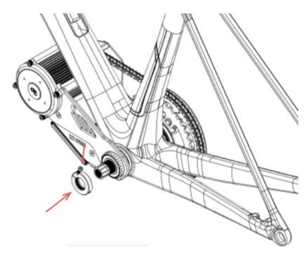
5. Install the motor hanger and place the rubber padding provided in between the motor and the frame.
