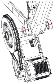
2. Line up the motor body with your frame at the bottom bracket and insert the right (drive) side of the motor into the frame's bottom bracket shell.
