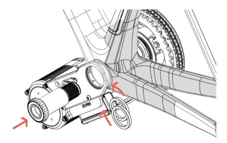
3. Insert the spindle from the right (drive) side. Note that you will need to line up the splines with the chainring assembly. If your spindle does not go through or comes to a hard stop before being fully inserted, rotate the spindle slightly and try again. Once the spindle is lined up, a soft tip hammer may also be used to get the spindle all the way through.
